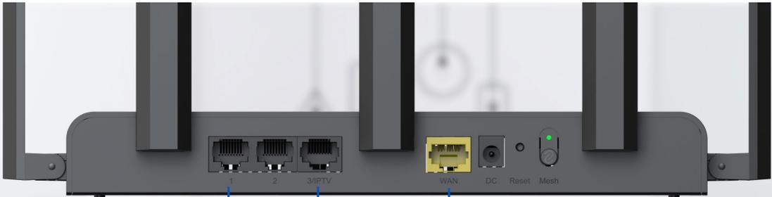
The image shows the back panel of a black Ruijie router. On the left, there are three Ethernet ports labeled 1, 2, and 3/PTV. On the right, there is a yellow WAN port, a DC power jack, a Reset button, and a Mesh button. Blue lines connect the WAN port to a label 'Gigabit LAN Port' and the three LAN ports to a label 'Gigabit WAN Ports'.
